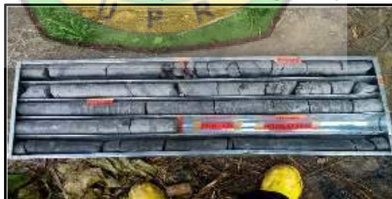
Gambar 4.12 Hasil Pengambilan Sample Bor Coring
